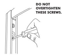
**CHECK THE DOOR** frame is level - each wallpost has 3 nylon adjustment screws. Turning these screws in an anti-clockwise direction forces the outer wallpost channel & frame away from the wall up to 15mm.
