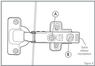
To make adjustment I tighten/loosen adjustment B. To make adjustment 2 simply turn screw A.
