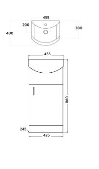
Dimensions (measurements in mm)
