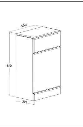
Dimensions (measurements in mm)
