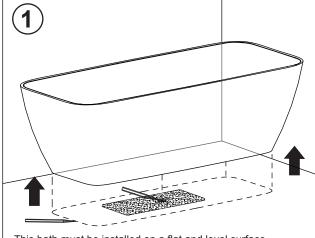
This bath must be installed on a flat and level surface. Remove any humps from the floor before installing. Under floor access required for plumbing of bath waste.
