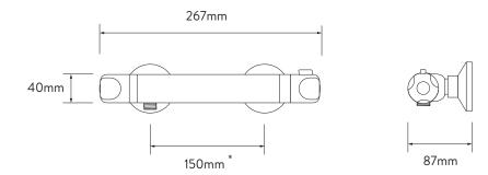
\*Pipe centres can be adjusted between 130mm-170mm using supplied elbows
