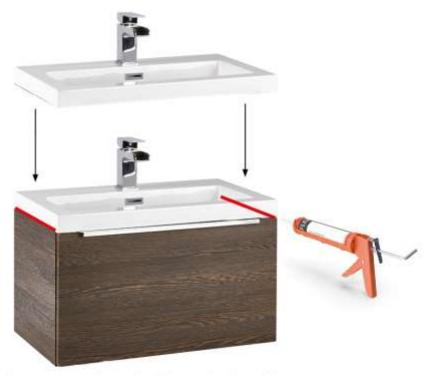
Silicone on top edge of the side panels only and lower basin on top of silicone to form a watertight seal
