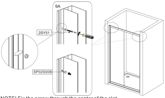
NOTE! Fix the screw through the center of the slot. This is necessary to allow enough room either side for the screw cover caps
