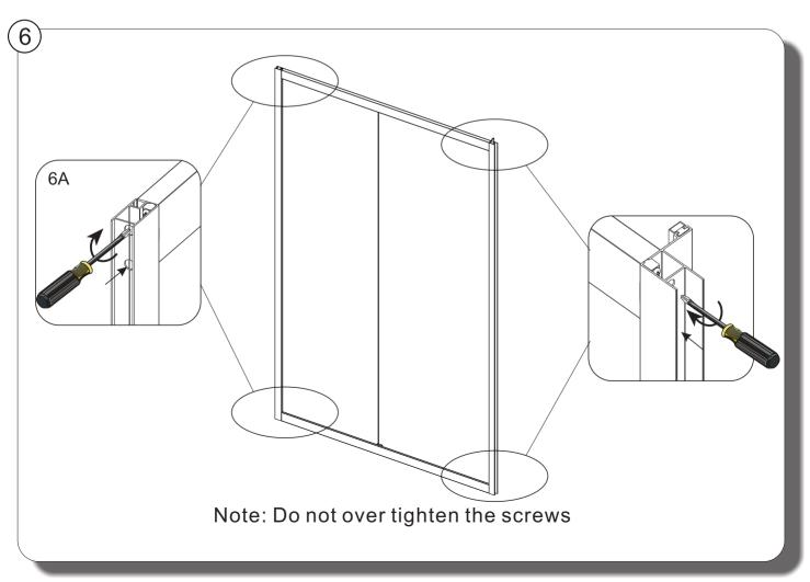
Tighten A12S0020 onto the fixed panel to secure the glass .
