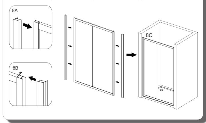
9 Lift the frame including wall profiles onto the tray and then fix your wall profiles to the walls using the fixing screws provided.
