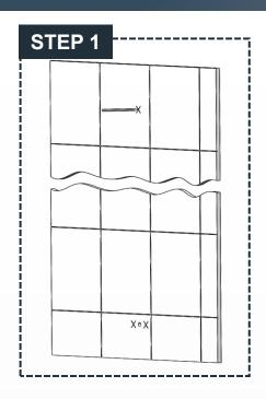
**STEP 1:** Select the desired position, then utilize a measuring tape to determine the distance between the center points of each wall bracket tube, and mark the location with a pencil.
