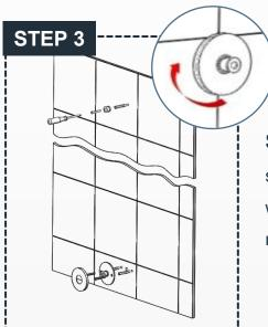
**STEP 3:** Insert one M4\*45 screw through the fixing block and two M4\*30 screws through the mounting seat and then secure them into the plastic wall anchors with an electric drill. Place the decorative cap onto the mounting seat and tighten it.
