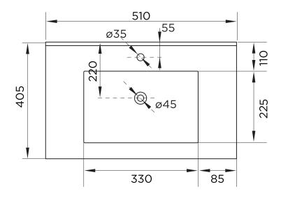
Diagrams not to scale All dimensions in mm tolerance of +/-5mm
