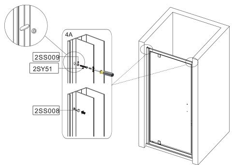
NOTE! Fix the screw through the center of the slot. This is necessary to allow enough room either side for the screw cover caps
