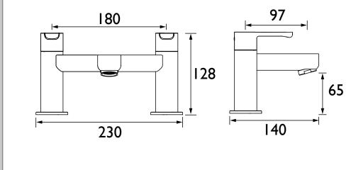
Flow Rates (I/min) System Pressure (bar) 0.2 0.5 5 1 2 3 NR BF C (mixed) 150.7 30.1 47.6 67.4 95.3 116.7 TECHNICAL BR DATA S D8
