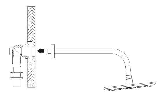
Wrap PTFE Tape around the thead on the wall arm and screw into the back plate elbow. Screw drench head onto the wall arm.
