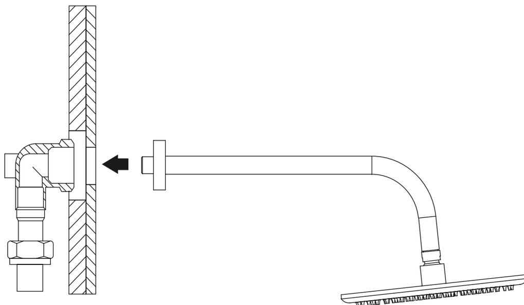
Wrap PTFE Tape around the thread on the wall arm and screw into the back plate elbow. Screw drench head onto the wall arm.
