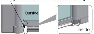
7. To change the handing of the stabilising bar **BSYS023**, unscrew wherethe arm attaches to the glass clamp and reverse. Place the stabilising bar onto the fixed panel. Mark the fixing point for the bracket to the wall. Use 6mm masonry bit, insert 1 wall plug **2SP12** and fix to wall with screw **2SY51**. Fasten the bracket to the glass keeping the washer on the outside of the glass. Attach cover caps to bracket. Fig 7.
