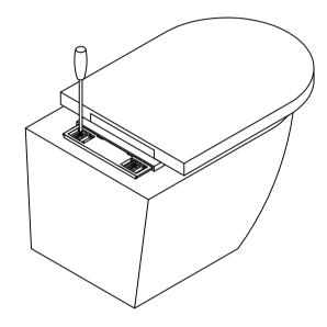
WITH THE FIXING PLATE AND BOLT SETS IN POSITION, SLIDE THE PLATE BACK INTO THE HINGE PLATE 5mm ONLY AS THIS WILL ALLOW ACCESS FOR TIGHTENING THE BOLTS.
