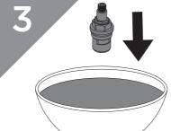
Place valves in a suitable solution and soak until fully de-scaled.
