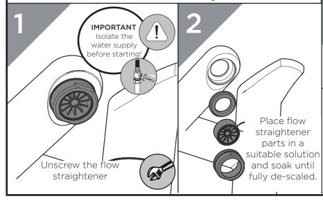
Reverse the maintenance steps to replace the flow straightener
