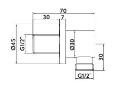
Dimensions (measurements in mm)
