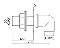
Dimensions (measurements in mm)
