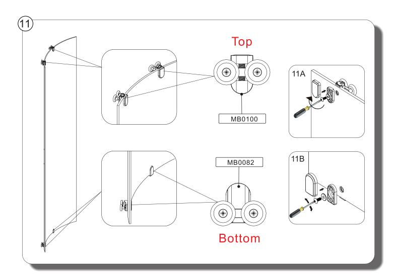
To fit your door panel first hang the top roller to support the weight of the glass panel. Push down the bottom roller fully and guide the roller into the bottom track.
