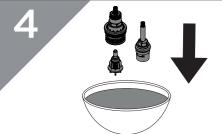
Remove any O-rings and soak all components in de-scaler and wash off in clean water. Examine all seals and replace if needed. Use WRAS approved silicon based grease on all seals.
