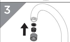
Replace the flow straightener, making sure the filter washer is in place.
