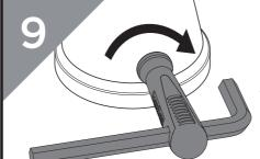
Thread the hexagonal key through the EasyFit tool and tighten the grub screws with an extra 1/2 turn.
