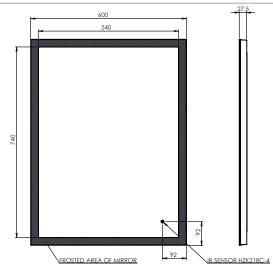
Diagrams not to scale.All dimensions in mm (tolerance of +/-5mm)
