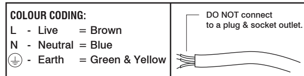
WIRING DIAGRAM - MAINS SUPPLY
