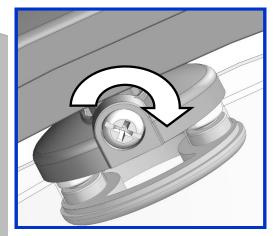
Adjust door heights until bottoms of doors just clear base of guide, doors are even & run smoothly. Adjust door angles so that magnetic seals hold door closed with no gaps. Turn adjusting screw clockwise to raise door.
