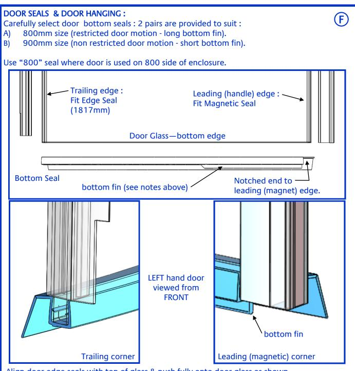
Align door edge seals with top of glass & push fully onto door glass as shown. Check magnetic seal orientation before fitting (aligned & attracting each other). Select appropriate bottom seal & push fully onto base (ensure soft 'drip' fin to inside of curve). Seals may be 'wetted' to ease assembly.
