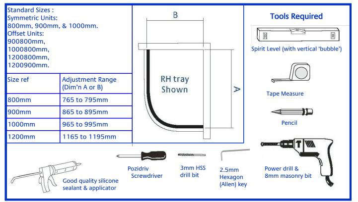
Lakes Offset Quadrant is fully reversible, so is suitable for fitting to right or left hand trays. Ensure tray is correctly levelled & that tray / wall (tile) joints are sealed & cured over entire length of tray sides (See Fig A) prior to fitting enclosure. DO NOT SEAL TRAY EDGES UPTO A FITTED ENCLOSURE !
