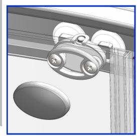
After adjusting, check that clamp screws are tight & fit covers to wheels
