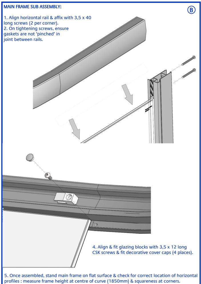
If required, loosen frame corner screws, adjust as necessary & re tighten.
