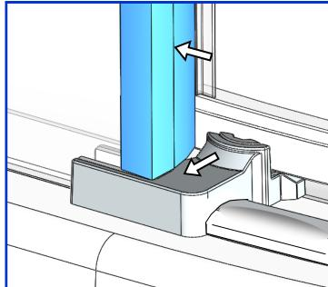
Stand edge seal on guide, then working from bottom to top, push edge seal fully onto fixed glass panel.
