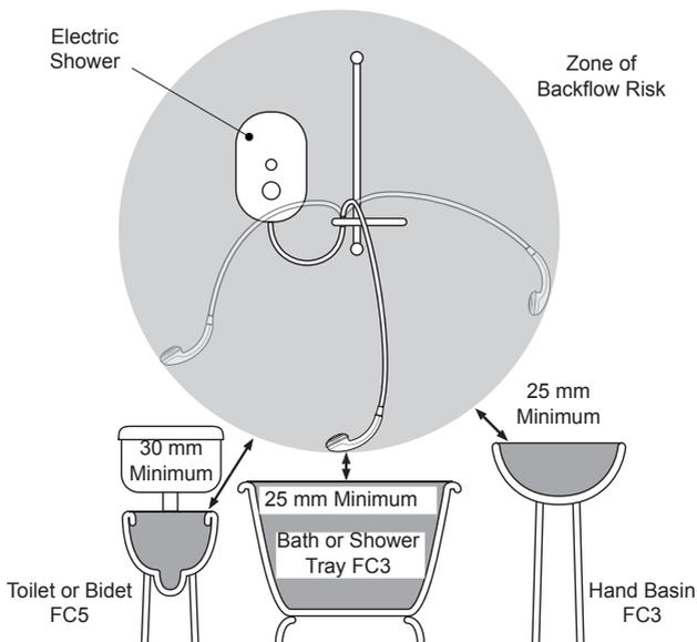
**Hose Retaining Ring (Integrated into soap dish) fitted and shower fittings fixed at a suitable height preventing dirty water backflow**
