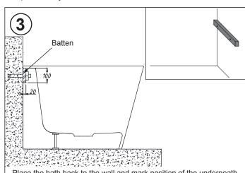
Place the bath back to the wall and mark position of the underneath of tap ledge. Screw a batten of 100x20mm treated timer to the wall horizontally to support the bath tap ledge. This ensure that the bath tap ledge will remain stable.
