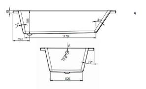
Dimensions (measurements in mm)
