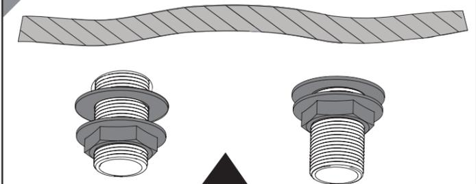
Secure the taps to the bath by using the washer and metal backnut below the bath.
