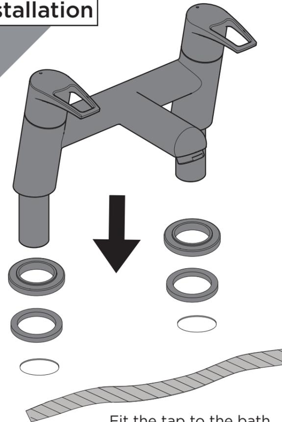
Fit the tap to the bath, ensuring the plinths are in place.
