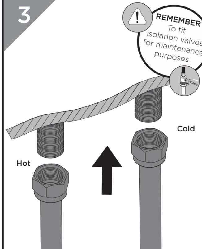
Connect the hot and cold water supplies to the threaded tails.
