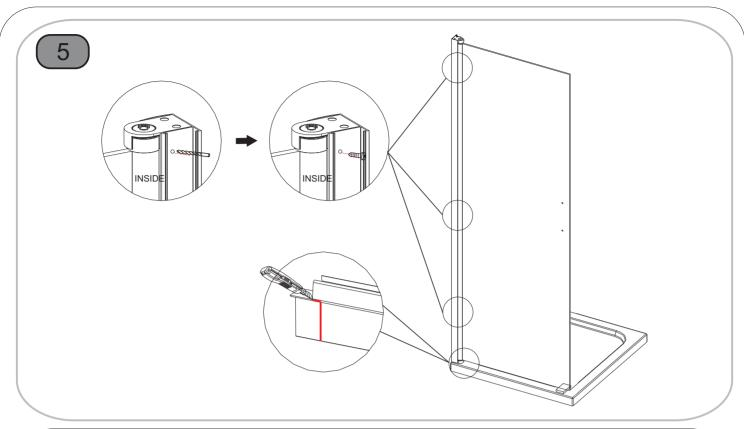
Note: If fitting as a shower wall skip to step 09 for sealing instructions. If fitting as a corner door skip to step 10.
