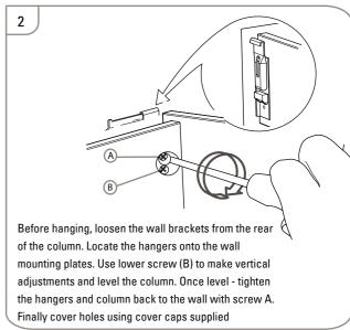
Note: - There are two sets of hangers on the back of the column. This allows the column to be hung so that the door opens in the desired direction.
