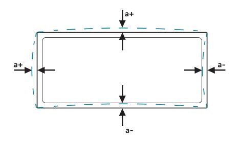
The flatness of the top surface of the outer rims is subject to the maximum tolerances shown in the table below in both directions (convexity and concavity).
