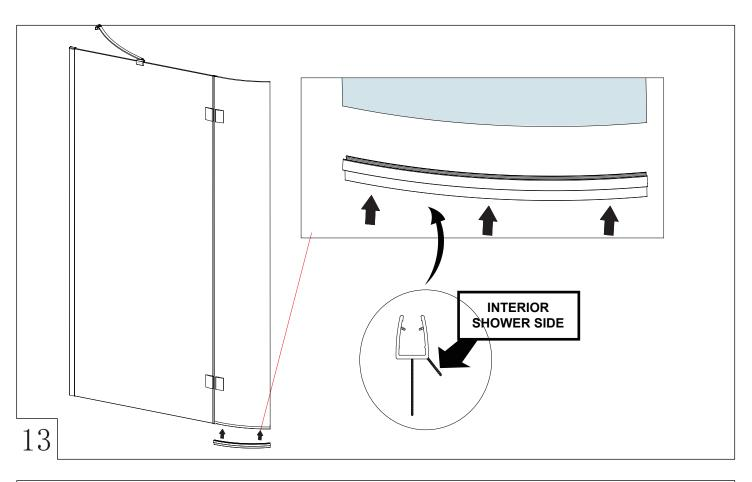
Before sealing make sure all surfaces are clean, dry and free from any residue such as grout. Use quality silicone sealant and applicator gun to finish the door.
