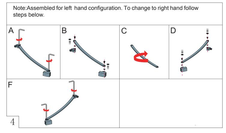
A.Position the bracing bar on the glass and against the wall.Make sure the bracing bar clamp is a minimum of 300mm from the edge and between 30-45 degrees to the glass.
