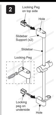
Using a suitable tool, push and hold down the locking peg through the hole in the slidebar support and pull off.
