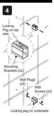
Remove and discard the existing mounting brackets, wall plugs and screws.
