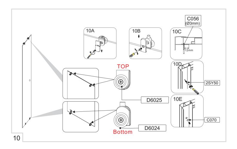
To fit your door panel firstly hange the top roller to support the weight of the glass panel. You can then leave your door panel hang making it easier to release your easy clean roller into the bottom track.
