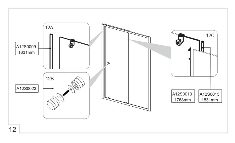
You can adjust the gaps between the door panel and the closing post by turning the adjustment screw in the top roller.
