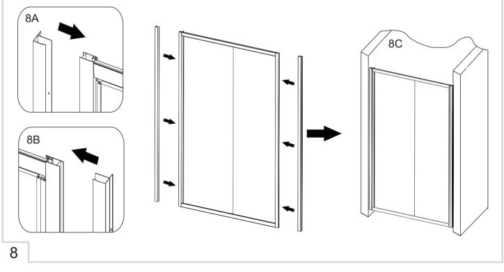
When the enclosure is between your two walls you can then fix your wall profiles to the walls using the fixing screws provided. Equalise the gaps on either side of the upright profiles and fix using 2SY50
