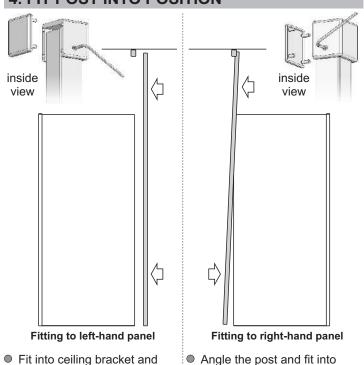
Secure post to ceiling bracket by tightening bracket grub screw with 3mm allen key provided and fit the bracket cover cap.
