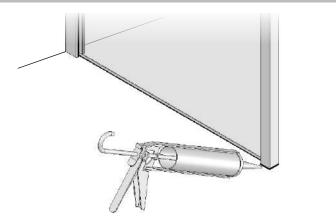
Apply silicone sealant to bottom of post to floor/showertray on the outside.
