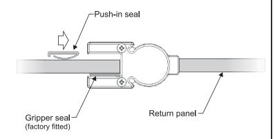
Fully insert push-in seal to secure channel to glass panel.
