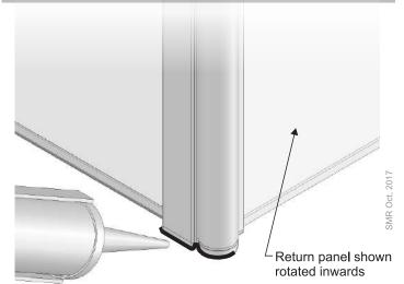
Apply silicone sealant around bottom cover cap to floor/showertray on the outside, as shown. DO NOT apply sealant around bottom cover cap on the inside of enclosure.
