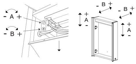
2.9 – When the cabinet is level, mark the hole on the lower section of the cabinet backboard (2.9). Take the cabinet off the wall.
