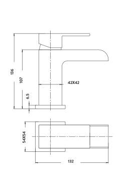
Dimensions (measurements in mm)
