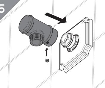
Push wall outlet fitting through wall plate. Secure in place with grub screw. Screw the shower hose (not supplied) onto the outlet ensuring the sealing washer is fitted.
