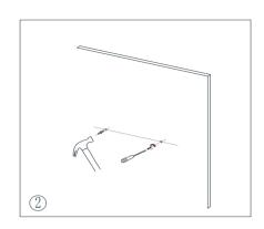
Insert the wall plug and mounting screw into the wall.
