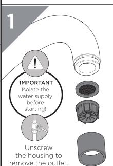
Check seals for damage. Soak using a suitable solution to de-scale.
