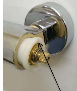
3. The Temperature Stop Lug and Cartridge Spline are now visible.
