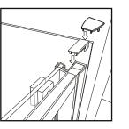
10 - Once you are happy that the installation is correct and that the doors are running smoothly, push the cover caps onto the top of the wall channels as shown, (smaller top cap first followed by the larger wall channel top cap).
