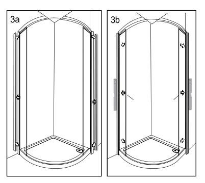
3a - Push the wall channels onto the edges of the assembly as illustrated and then position the assembly onto the shower tray as shown (roughly 10mm from the outer edge of the tray).
