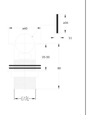
Dimensions (measurements in mm)
