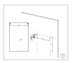
Measure the distance of the mounting hole, Drill holes with a suitable sized drill.
