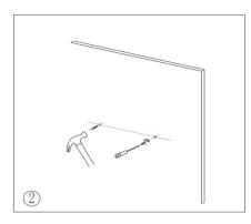
Insert the wall plug and mounting screw into the wall.
