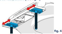
**Note:** Rotate the plastic studding 180° to allow for maximum or minimum hole alignment within the slider bracket
