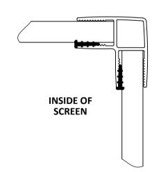
FINALLY FIT THE WEDGE SEALS (ITEM 17) INTO THE CORNER PROFILE AS SHOWN ABOVE. STARTING AT THE BOTTOM, PUSH THE SEAL ALONG THE LENGTH OF THE PROFILE. A WOODEN BLOCK CAN BE USED TO AID FITTING. TRIM OFF ANY SURPLUS SEAL AT THE TOP SO ITS EVEN WITH THE PROFILE.
