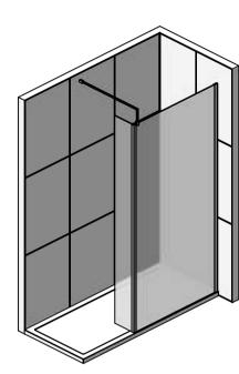
SLIDE THE RETURN GLASS PANEL (ITEM 16) INTO THE CORNER PROFILE (ITEM 15) ENSURING ITS FULLY INSIDE.
