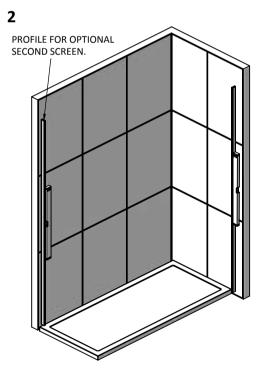
POSITION THE WALL PROFILES ON THE TRAY IN A SUITABLE POSITION. MAKE SURE THEY'RE TRUE WITH A SPIRIT LEVEL, THEN MARK THROUGH THE FIXING HOLES WITH A PENCIL. REMOVE PROFILES THEN DRILL AND PLUG THE WALL (ITEM 12). NOW FIX THE WALL PROFILE IN PLACE USING ITEM 11.
