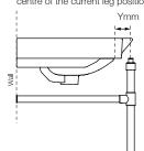
Remove the side bar from the joint and cut distance Y on both bars.
