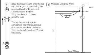
Cut distance X from the base of the leg. Cut the same distance on both legs.
