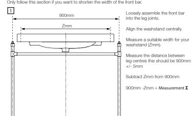
Remove the front bar from the leg joints and cut Measurement  $\Sigma$  on one side.
