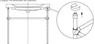
Once the washstand is aligned and level, mark out and drill the pilot holes using a suitable drill bit. Insert the wall / floor plugs.
