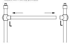
Adjust the height of the front bar and side bars by sliding the leg joint up and down until you have the desired height.
