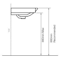
Ensure the basin is firmly secured to the wall using appropriate basin fixings before proceeding with the installation of the Washstand,
